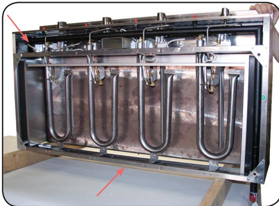
2. Remove the back and underneath panels of the griddle revealing the innards of the griddle. Make sure the griddle is SECURE while standing in place for the adjustments. Safety First.
