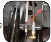
9. Determine the correct injector size for the corresponding gas from the rating label. Replace with the correct size injectors.
