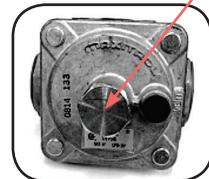
7. Before installing the included convertible regulator, unscrew the octagon cap. You can read (NAT) on the plastic insert attached to the head of the cap; flip it over and snap back in place.
