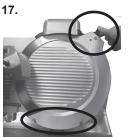
11. the knife and the knife ring guard. While holding the cloth between the knife and the ring guard, work it along the inside surface of ring
