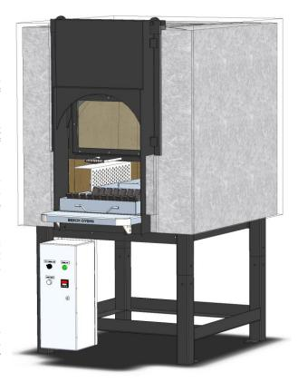
The oven can be installed within 75mm (3") (including 50mm (2") of insulating wool and 25mm (1") air gap) of non-combustible material (check local building and fire codes). The oven exhausts through a spigot above the oven mouth. The oven must be vented in accordance with local and/or national codes. Refer to "Duct Design Options" or for more information, refer to the Installation and Operation Manual located on our website <a href="https://www.beechovens.com">www.beechovens.com</a>
