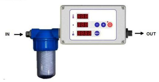
The accessories to be used for fixing the equipment are supplied to fix the meter to the wall. First, fix the meter to a flat wall, in the position shown, then connect the water hoses and then the power cable. If the meter is not fitted in a horizontal position, the precision of the measurement is reduced.
