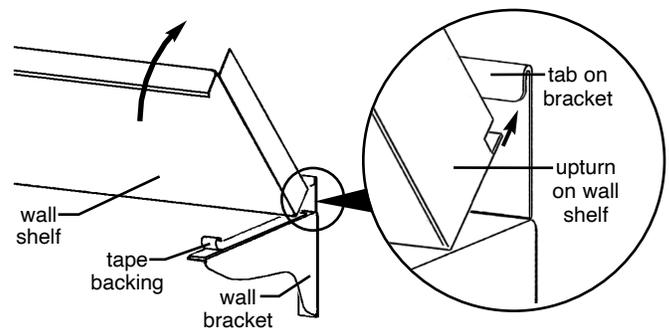
Rear upturn of wall shelf hooks under tab of each bracket.
