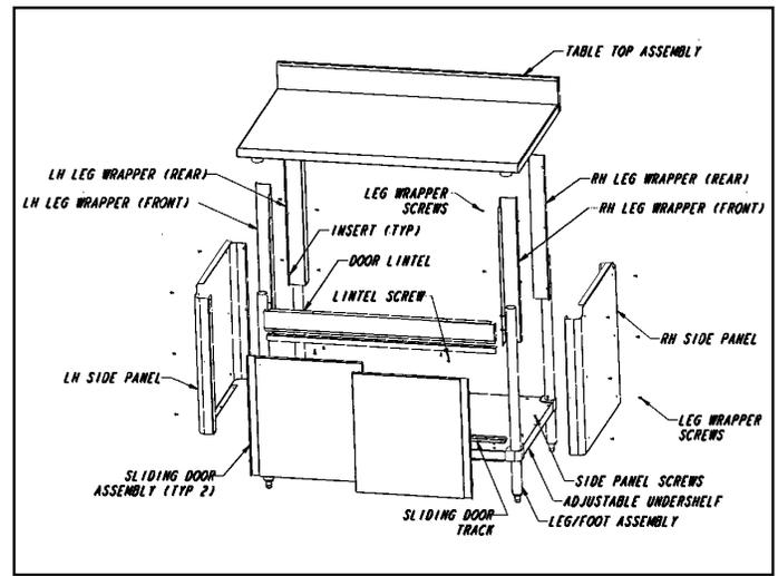
(1) With set screws\* provided, attach leg/foot assemblies to the adjustable undershelf. Leave 6" from the bottom of casting to bottom of leg (as shown).
