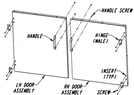
(11) Install (female) hinges to side panel inserts (female adapter should be on the bottom).
