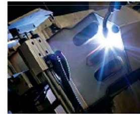
Robotic welding is precise, virtually eliminating leaks.
