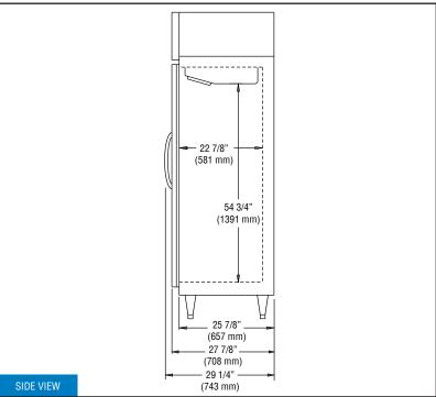
**IMPORTANT NOTE:** If the cabinet is located directly against a wall and/or under a low ceiling, a minimum clearance of 12" is required on top and 3" on sides and rear.
