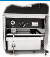
On-Board Oil Filtration System: Designed to complete a filter cycle in 5 minutes. Uses disposable paper filter media, or optional reusable steel mesh filter screen. Provides for 1-step draining, oil filtering, and vat cleaning. Turn a single valve to refill vat with reconditioned oil. When used properly, can increase useful life of oil by at least 50%.
