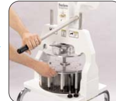
Figure 3: While holding the Handle down with one hand, use your other hand to rotate the Head Assembly 1/4 turn until the Head Assembly releases.
