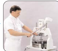
Figure 2: Push downward on the Trip Lever and hold while pulling the handle down which will separate the Head Assembly from the Trip Plate.
