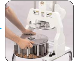
Figure 4: Return the Handle to the upper position and remove Head Assembly for cleaning or interchange with Optional Head Assembly.
