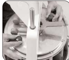
Figure 1: Remove pan, completely loosen both Black Knobs. Do not Drop the Divider Head as damage may occur!
