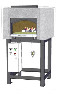
The oven can be installed within 75mm (3") (including 50mm (2") of insulating wool and 25mm (1") air gap) of non-combustible material (check local building and fire codes). The oven exhausts through a spigot above the oven mouth. The oven must be vented in accordance with local and/or national codes. Refer to "Duct Design Options" or for more information, refer to the Installation and Operation Manual located on our website <a href="https://www.beechovens.com">www.beechovens.com</a>
