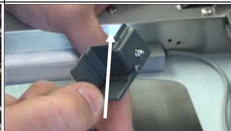
Fig. Q 12) With the wire notch facing down, replace the bottom bracket.
