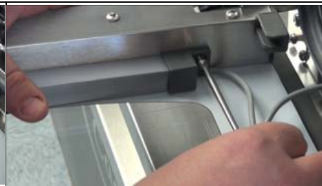
Fig. F 6) With Phillips head screwdriver, unscrew and remove both light cover brackets. Figs. E-F-G.
