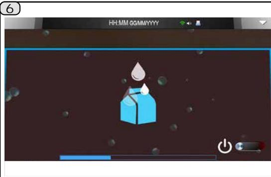
On the touch screen the milk circuit wash symbol appears, and remains visible for the entire cycle. This stage ends when the progress bar below is filled.
