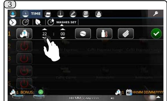
The user can only change the wash times according to their needs. When the operation is done, confirm the selection with the
