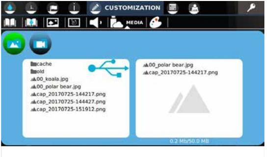
Select the desired image file from the machine memory and push the
