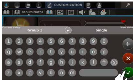
Group names can be changed by pressing the name itself. An alphanumeric keyboard will appear. Enter the desired text and confirm by pressing the
