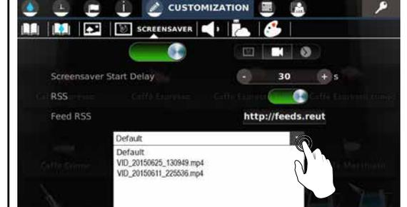
The screen saver can be customised using personal videos. Press the key to show available videos and press the name of the desired file (see the media section for how to load files on the machine).
