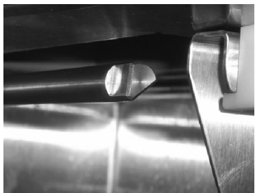
Figure-10: Door Alignment Arrow
