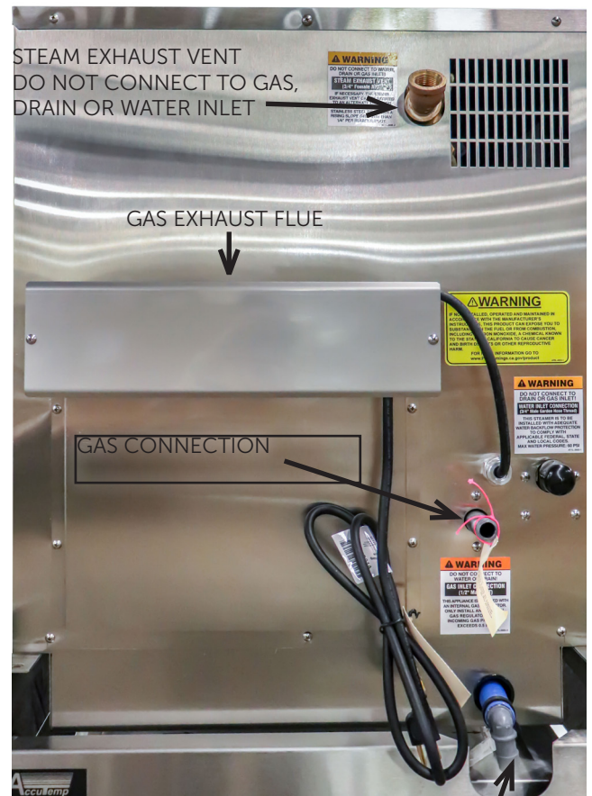
DRAIN CONNECTION CONNECTED STEAMERS ONLY
