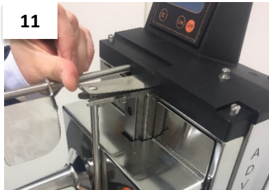
11. Remove the knife by lifting the fastening tab up top and then lifting the knife out of its anchorage.
