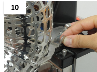
10. Unclamp the locking lever and remove the fruit supply tunnel.
