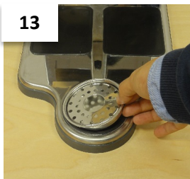
13. Remove the drip cup and the drip tray.
