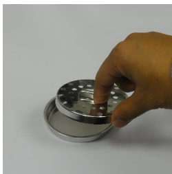
13. Remove the drip cup and the drip tray.
