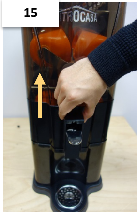
15. Remove the tap housing by pulling it up.
