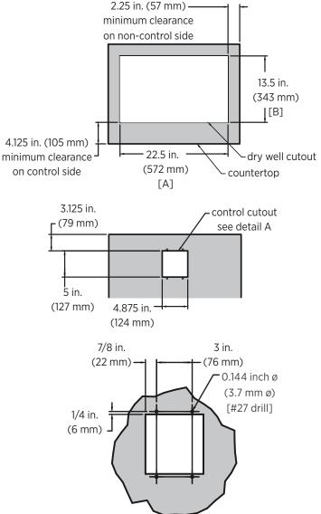
The unit's overall depth is 12.125 inches (308 mm) will sit approximately 11.75 inches (298 mm) below the counter surface depending on counter thickness.
