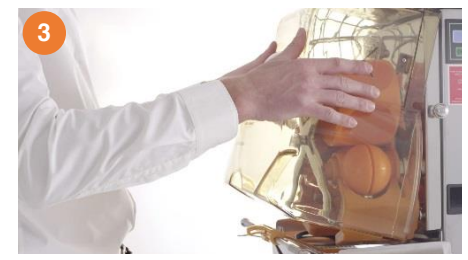
3. Unscrew front cover screws and remove front cover. CAUTION! HANDWASH ONLY!
