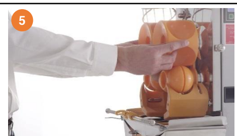
5. Remove upper pressing elements.
