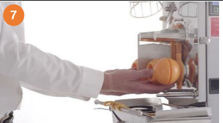
7. Remove lower pressing elements.
