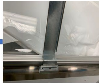
Lid locking bar assembly Then slowly move the bar towards the lid's inclined surface having a center of rotation at bottom hinge and lid handle
