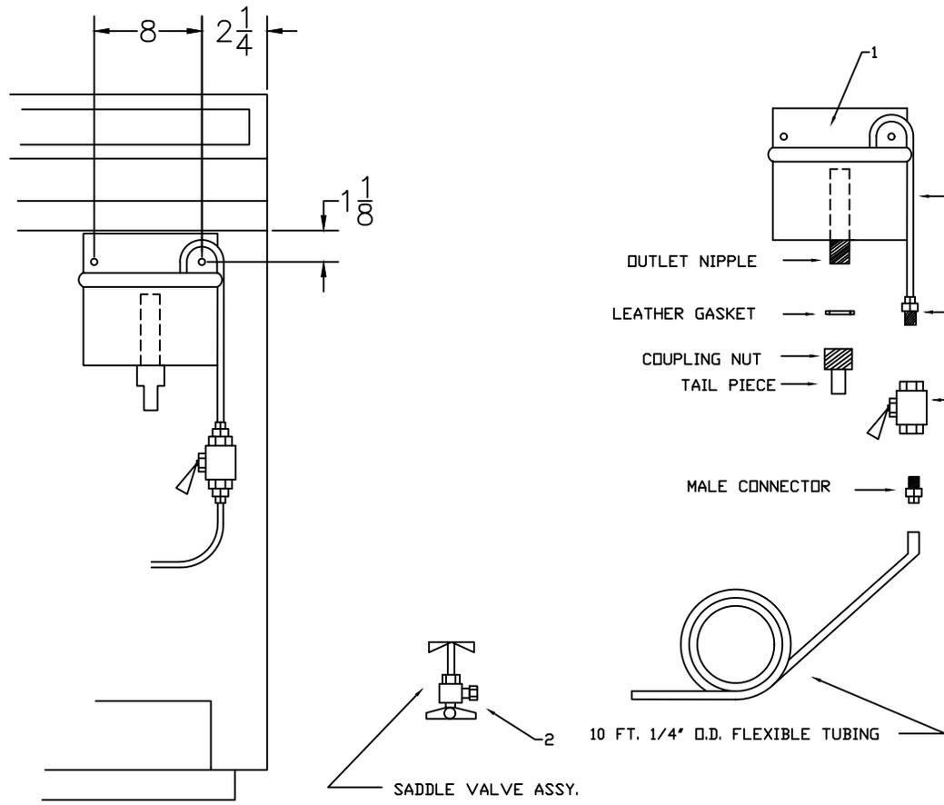
1- ATTACH DIPPER WELL TO CABINET WITH (2) 8"x3/8" SIMIS. SHUT OFF MAIN VALVE TO WATER SUPPLY AND RELEASE THE PRESSURE BY OPENING ANY SPIGOT IN THE SYSTEM. DRILL 1/4" DIAMETER HOLE IN THE WATER LINE ON BOTTOM SIDE OF PIPE.
