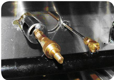
2. Unscrew bolts and pilot valve, then remove the manifold.
