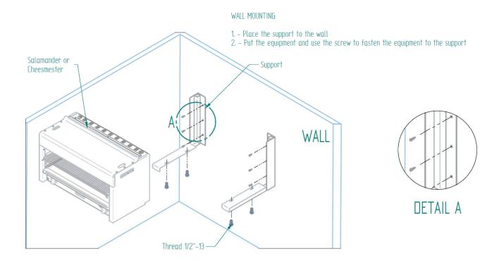
2. - Put the equipment and use the screw to fasten the equipment to the support.
