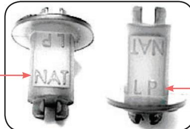
L.P. Position of insert. Regulator is now converted to L.P.
