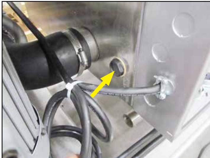
Fig. 11 - Detergent Sensor provided in side of wash tank
