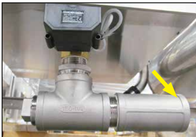
Fig. 6B - Drain connection
