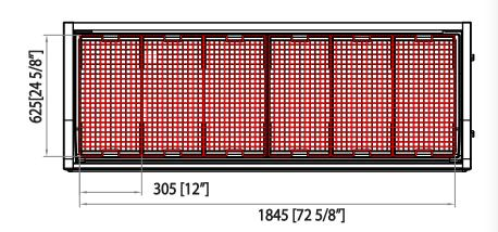
Basket 6 Capacity 24.72 Cu.Ft. Doors 2 Refrigerant R-290 -10°F ~ 0°F Sliding Easy Maintenance Condensing Unit 9.8 ft long (3m) flexible three Connection wire cord with modeled plug HP 3/4 Voltage 115V/60Hz 3.8 **Amps** NEMA Config. NEMA 5-20 Lighting Interior LED lighting
