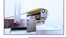
Pop-Up Conveyor Rollers, Large Access Panels, and Removable Working Tables Allow Easy Cleaning and Maintenance
