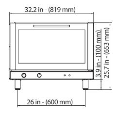
\* Oven must be installed a minimum of 19.7" (500 mm) from any significant source of heat and/or grease (for example: fryers, burners, kettles, open flames. etc.)
