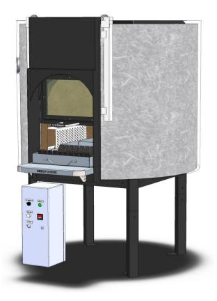
The oven can be installed within 75mm (3") (including 50mm (2") of insulating wool and 25mm (1") air gap) of non-combustible material (check local building and fire codes). The oven exhausts through a spigot above the oven mouth. The oven must be vented in accordance with local and/or national codes. Refer to "Duct Design Options" or for more information, refer to the Installation and Operation Manual located on our website <a href="https://www.beechovens.com">www.beechovens.com</a>
