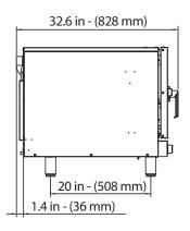
\* Oven must be installed a minimum of 19.7" (500 mm) from any significant source of heat and/or grease (for example: fryers, burners, kettles, open flames. etc.)
