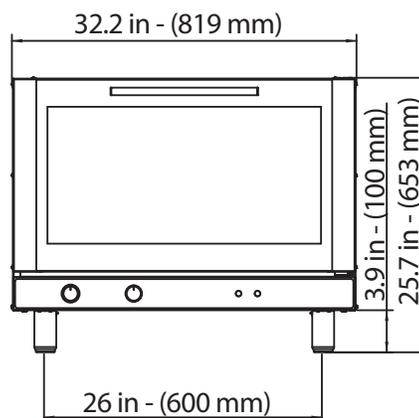
\* Oven must be installed a minimum of 19.7" (500 mm) from any significant source of heat and/or grease (for example: fryers, burners, kettles, open flames, etc.)
