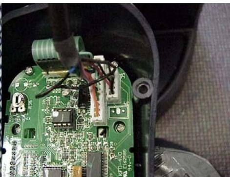
**Figure 6.** Wiring harnesses on rear of panel.
