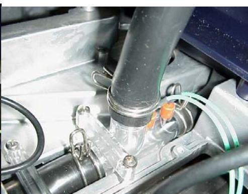
Figure 20. Drain sensor.
