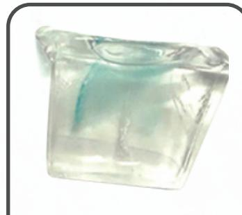
Turbulent water over the grid cell design traps air and impurities causing soft, cloudy ice that melts faster.
