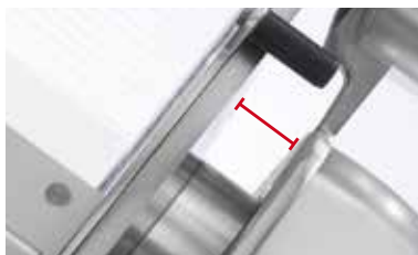
Increased gap between blade and machine body
