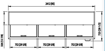
3 Doors Capacity 31.3 Cu.Ft. 6-pack of 12 oz Bottles 103 6-pack of 12 oz Cans 180 **Dividers** 5 Refrigerant R-290 **Temperature** 33°F ~ 39°F Range Sliding Easy Maintenance Condensing Unit 9.8 ft long (3m) flexible three Connection wire cord with modeled plug HP 3/8 Voltage 115V/60Hz **Amps** 3.5 NEMA Config. NEMA 5-15 Lighting Interior LED lighting
