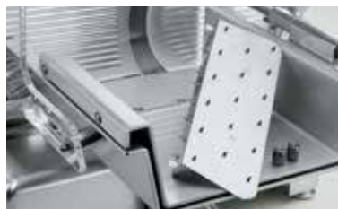
Double-feed carriage specially designed for fresh meat Removable product pusher
