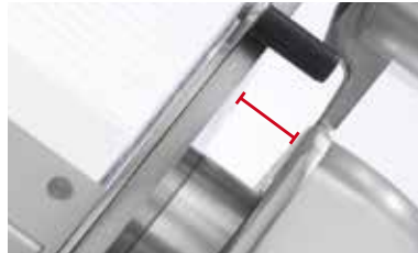
Increased gap between blade and machine body
