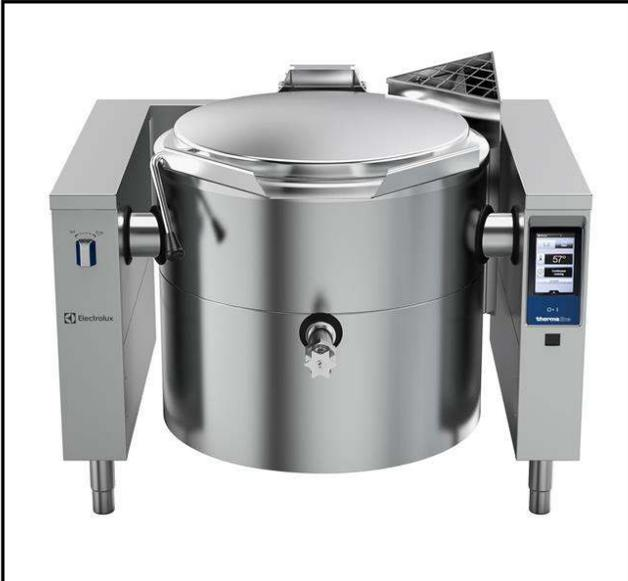
**587040 (PBOT10GCWF)** Touchline Tilting Kettle, gas, 26 gallon (100 Lt) capacity, stainless steel construction, full jacket, safety valve, safety thermostat, motor assisted tilt, 2" tangent draw-off valve, 71652 BTU
