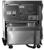
On-Board Oil Filtration System: Designed to complete a filter cycle in 5 minutes. Uses sustainable stainless steel mesh filter screen. Provides for 1-step draining, oil filtering, and vat cleaning. Turn a single valve to refill vat with reconditioned oil. When used properly, can increase useful life of oil by at least 50%
