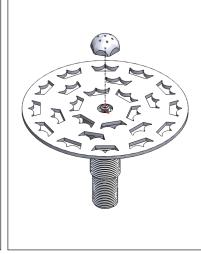
(OPTIONAL) If the stainless plate height needs to be higher, use the optional hard plastic black spacer. When checking to see if the additional spacer is required, it is important to include the rubber seal washer that is required for the installation step #4 for required height.
