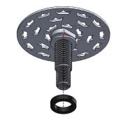
Place rubber sealant washer on the threaded section and install the complete glass rinser into the glass rinse station you are working on. A 7/8" hole is required for installation in new applications.
