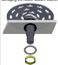
Install the plastic straight water line connector on threaded section and tighten properly. Thread sealant is not required on this fitting.
