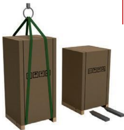
Figure 4 - Loading / unloading and transport of the machine
