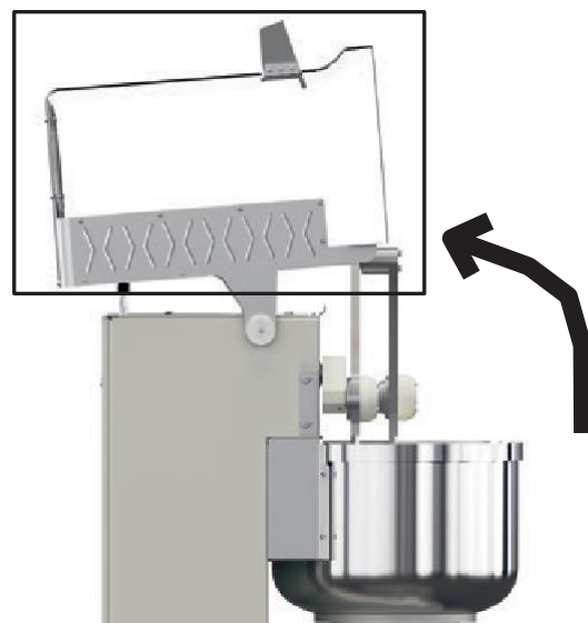
Figure 36 WEEKLY CLEANING Safety protection (internal)
