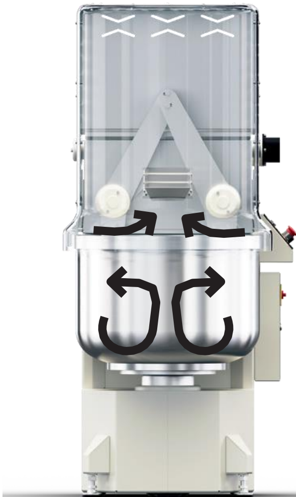
Figure 27 Motion of the utensil arms
