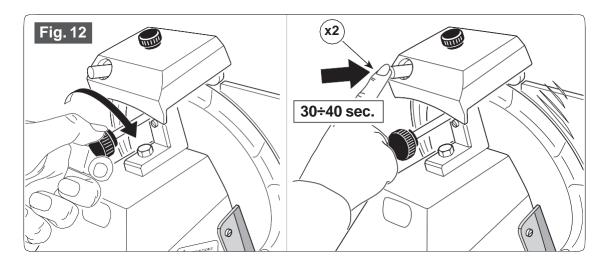
5. Ascertained the formation of burr, operate the switch (1) for 3/4 seconds again by pressing the buttons (x2 and x3) at the same time;
