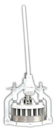
Table top model Dough Divider easily divide and evenly cut into 30 individual pieces from as little as 1.16 oz up to 3.5 oz each. SKYFOOD's DMS-30 will take variable quantities of dough compressing and cutting the dough into identical pieces that can be taken directly to the next process. Simply put in desired amount of dough (from 2.2 up to 6.6 lb), pull handle and individual dough pieces are ready to use. One of the most valuable tools in precision baking today.
